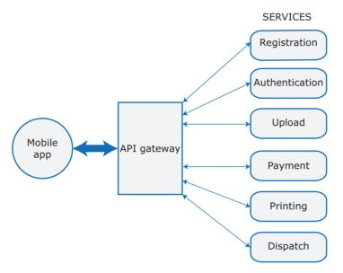
Figure 6.5 A microservices architecture for a photo-printing system
