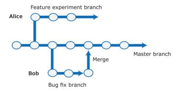
that file (Figure 10.7). Alice is working on a new experimental feature, and Bob is working on a bug fix.
