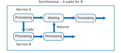
Figure 6.7 Synchronous and asynchronous microservice interaction
