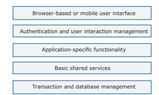
Figure 4.10 A generic layered architecture for a web-based application
