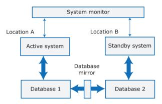
Figure 5.15 Using a standby system to provide resilience
