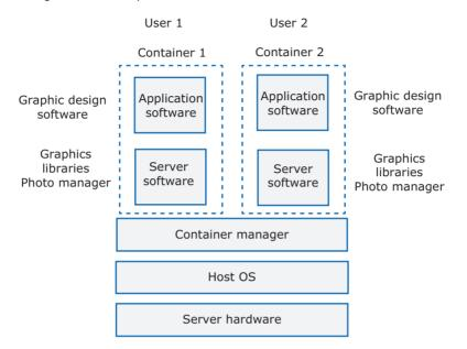
Figure 5.3 Using containers to provide isolated services
