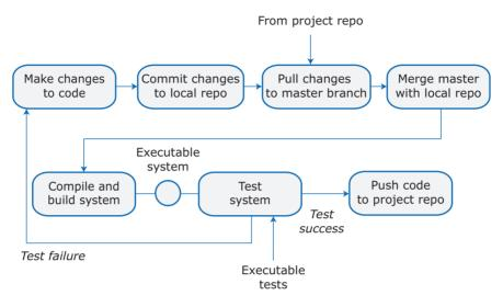
The squares in Figure 10.9 are the elements of a continuous integration pipeline that is triggered by a repository notification that a change has been made to the master branch of the system.
