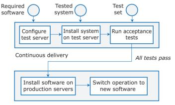
Figure 10.13 Continuous delivery and deployment
