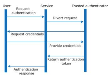
Figure 7.5 is a simplified description of the sequence of actions in a federated identity system.
