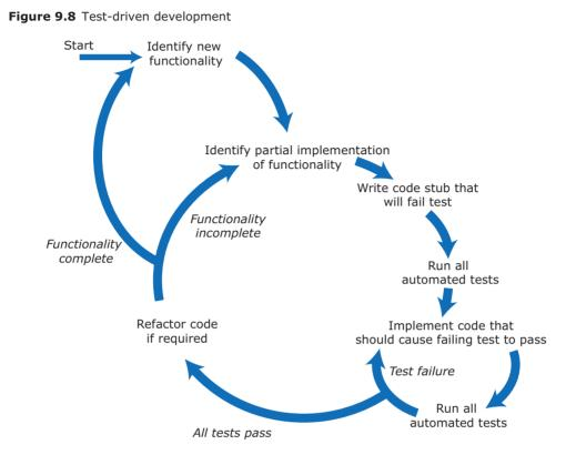
with any incremental development approach. Figure 9.8 is a model of the test-driven development process.
