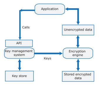
Figure 7.15 Using a KMS for encryption management
