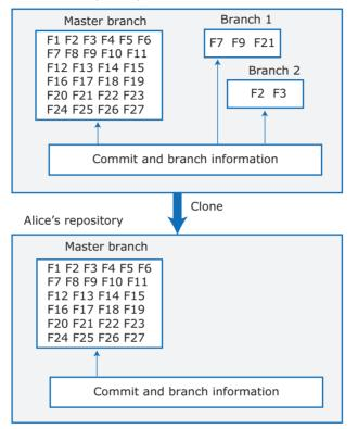
see that two branches have been created in addition to the master branch. When users request a repository clone, they get a copy of the master branch that they can work on independently.
