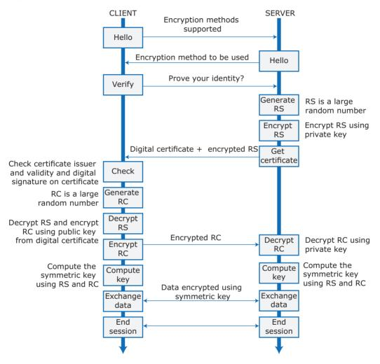
Figure 7.13 Using symmetric and asymmetric encryption in TLS
