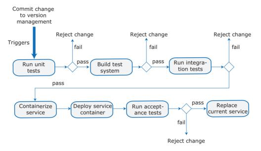
Figure 6.16 A continuous deployment pipeline
