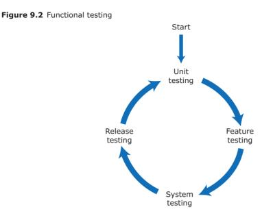
Software testing is a staged activity in which you initially test individual units of code (Figure 9.2 and Table 9.2). You integrate code units with other units to create larger units and then do more testing. The process continues until you have created a complete system ready for release.
