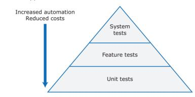
Figure 9.5 The test pyramid
